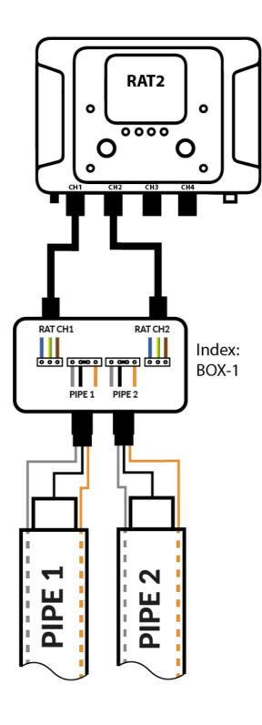
THE WAY OF CONNECTING RAT-2 DETECTOR TO THE ALARM WIRES USING BOX-1 INSTALLATION BOX IN RESISTANCE SYSTEM.
